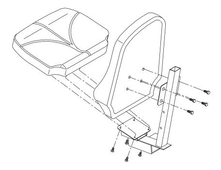
Connect back pad to seat support bracket using: Qty 4 - Allen Head Screw
